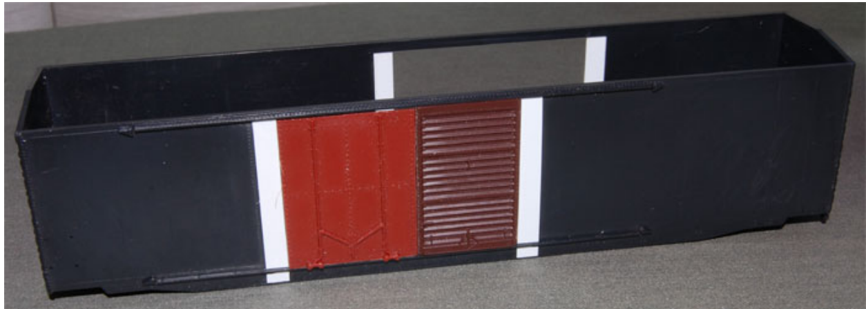
(above) The Front Range 50' double-door boxcar has a shouldered door opening to permit plug doors to be mounted flush with the side of the car. Begin the conversion by inserting a piece of Evergreen #128 .020X.188 styrene strip the length of the vertical edges on both the left and right sides of the door opening.
